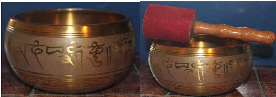
**Figure 3.** On the left the Tibetan bell used in the experiment, and on the right the bell and the drum stick to produce the sound. The emitted frequency is about 330 Hz.
